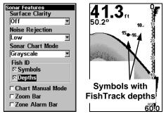
Sonar Features menu with Fish I.D. Depths selected (left). Sonar Page showing Fish I.D. symbols and FishTrack depths turned on (right).
